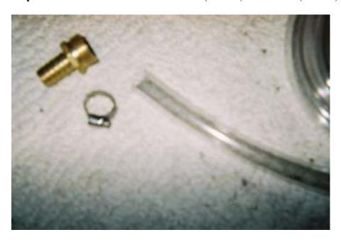
Before inserting the male barb into the hose, put the clamp on the hose. Then insert the male barb into the hose until it is fully inserted. Next, position the hose clamp (Part #2)
