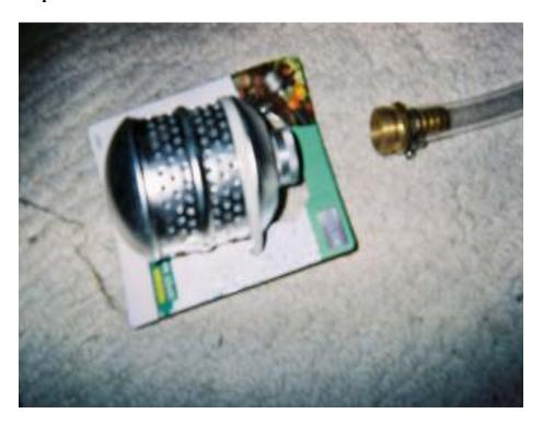
Screw the bubbling garden soaker (Part #4) onto the 5/8" brass hose barb. Hand tighten.
